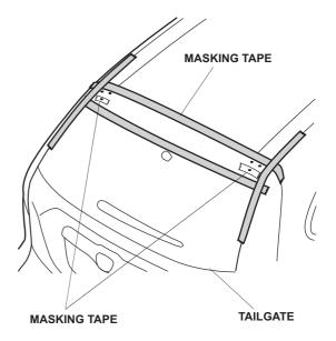
7. Open the tailgate. Apply masking tape over the ends of the taillight housing. Close the tailgate.
