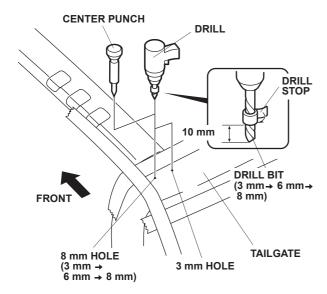
Repeat the steps 8 to drill the tailgate on the right side of the vehicle. Remove any burrs from the edges of the holes using a file, and apply touch-up paint to the edges. Allow the touch-up paint to dry.
