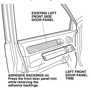
15. Repeat steps 12 through 14 to install the door panel trims for the remaining three doors.
