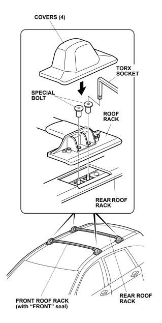
5. Reinstall the four covers on the front roof rack.
