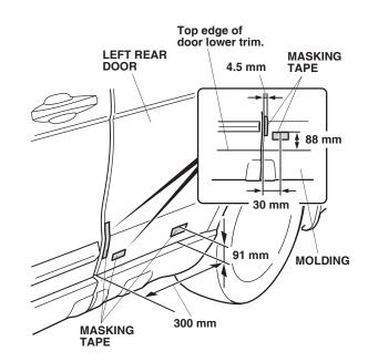
Peel back 1-1/2–2 inches of the adhesive backing, and tape them to the front of the rear body side molding. Remove the front and rear adhesive backings.
