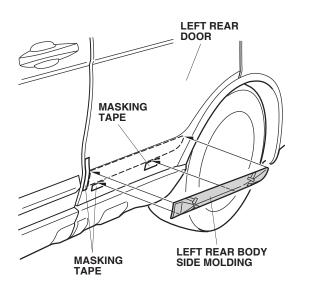
10. Position the left rear body side molding on the left rear door, aligning it with the masking tape you attached in step 7.
