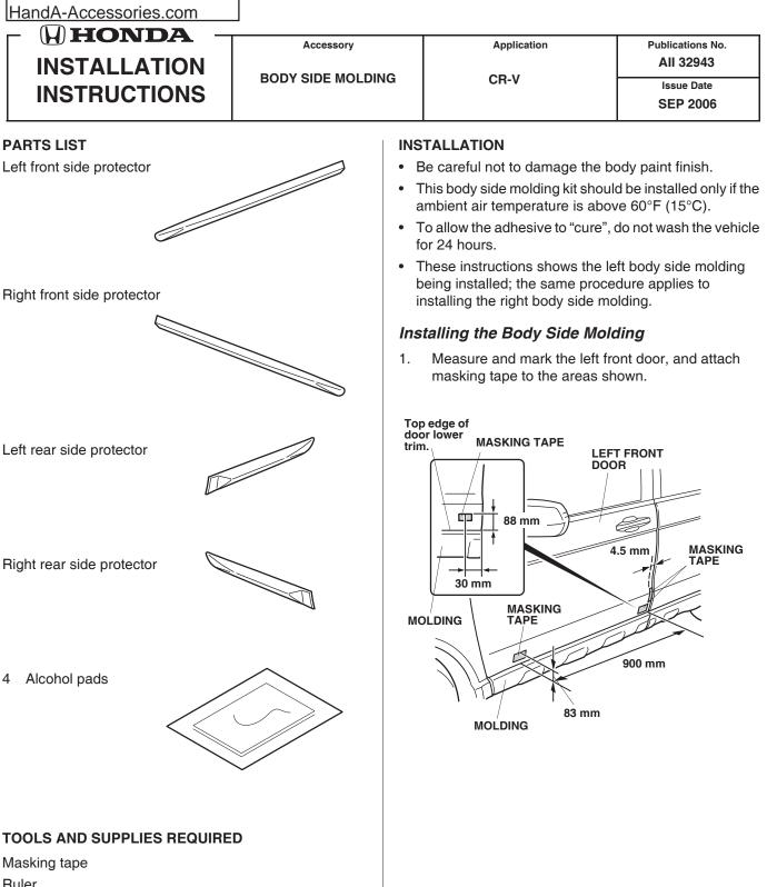
Ruler Isopropyl alcohol Shop towel  Peel back 1-1/2–2 inches of the adhesive backings, and tape them to the front of the body side molding. Remove the front adhesive backing.
