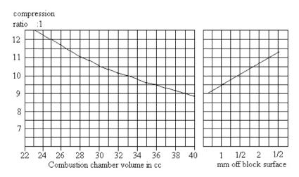
This graph shows the relationship between combustion chamber volume and the compression ratio.
