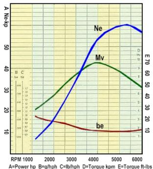
Ne=Power, DIN Mv=Torque be=Fuel consumption per hph
