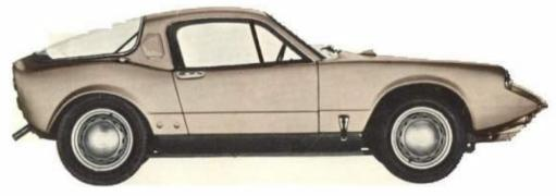
Front-wheel drive ... of course Sonett has front-wheel drive, all Saabs do — always have — for perfect traction, sure footed stable and SAFE driving. And streamlining ... the best — the air resistance rating is only 0.35.
