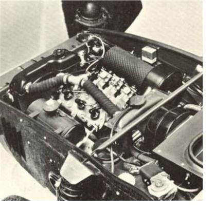
Saabs have shown they can take it, and so can Sonett with extra strong side beams, a box-type bulkhead behind the seats and built-in rollbar. The low, light body is made of fiber glass in only five sections. The whole front folds upward for easy access to the three-carburetor engine, the automatic oil injection system, or the thermostatcontrolled fan.
